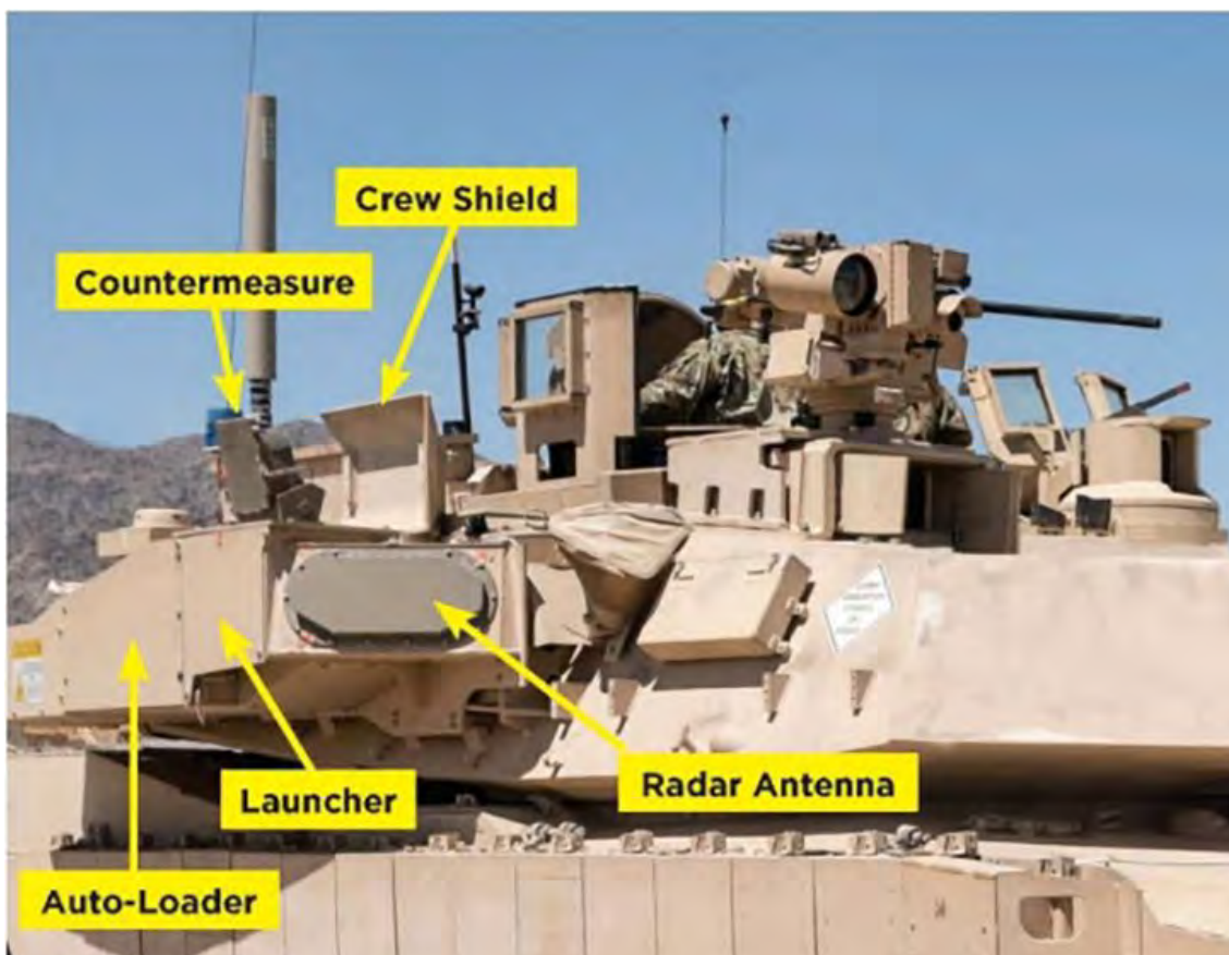
TROPHY integration on M1A2 used turret-side mounted modules, adapted from those deployed on IDF Namer and Merkava Mk4. Photo: Leonardo
