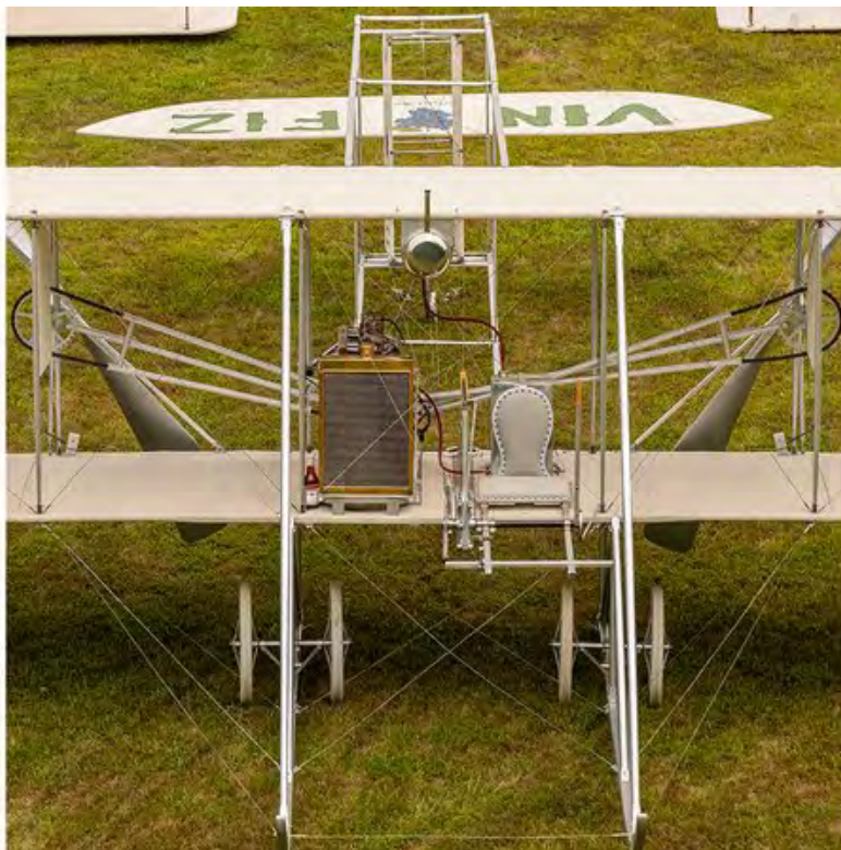
The 1911 Model EX (a reproduction of Cal Rodgers’ Vin Fiz, the first airplane to fly across the U.S.) shows the unusual—for the Wrights—rectangular radiator. (Dane Penland)
