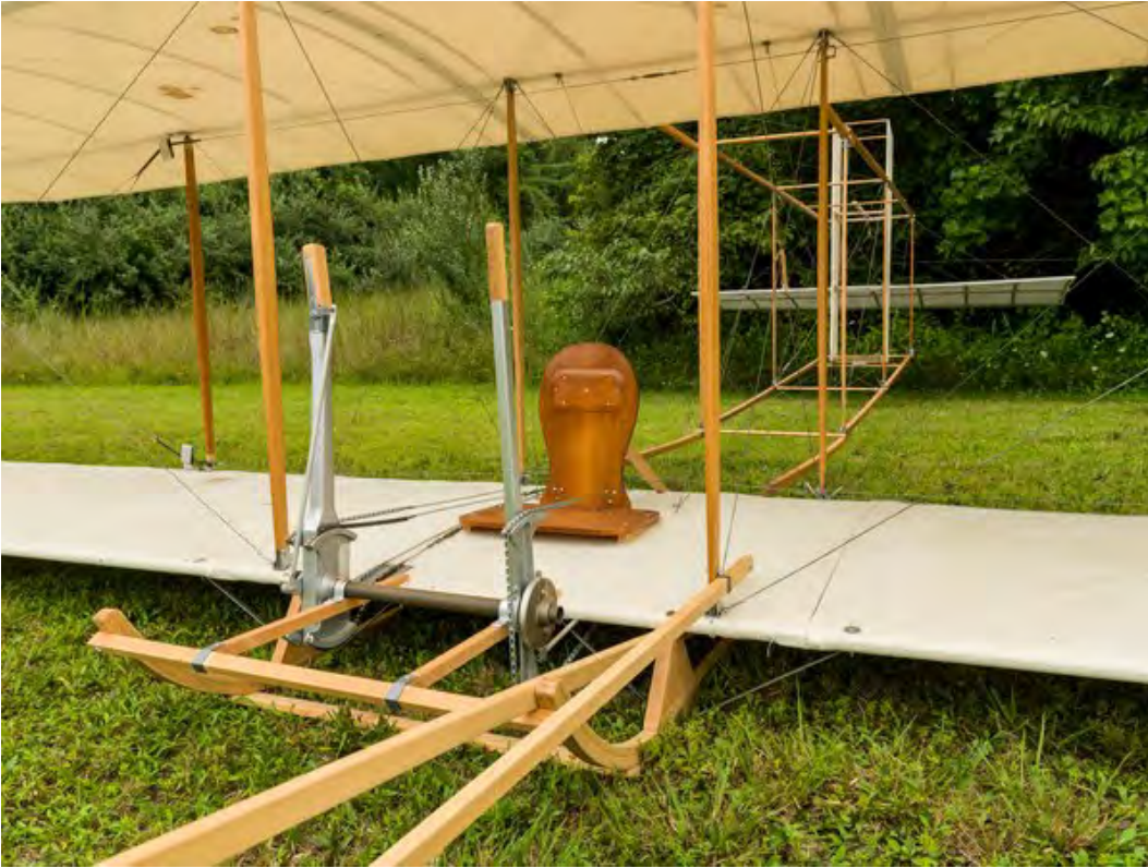
A close-up of the 1911 glider, which Orville used in experiments at Kitty Hawk. His diary entry for October 18, 1911, reads: "Made several glides. In last one, machine turned around in spite of all I could do and ran into hill, turning over. Broke both left wings and rear horizontal surface." (Dane Penland)
