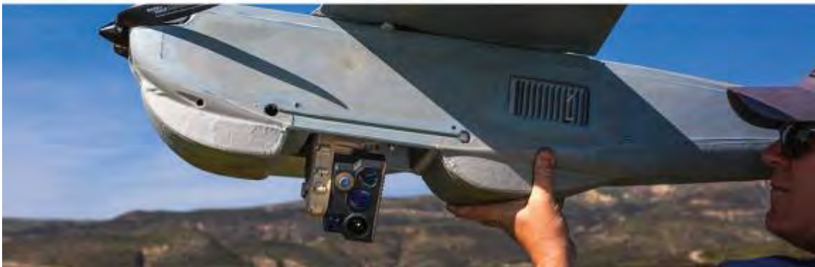
Puma's new Mantis i45 gimbal packs multiple sensors into a waterproof, retractable unit. Credit: AeroVironment
