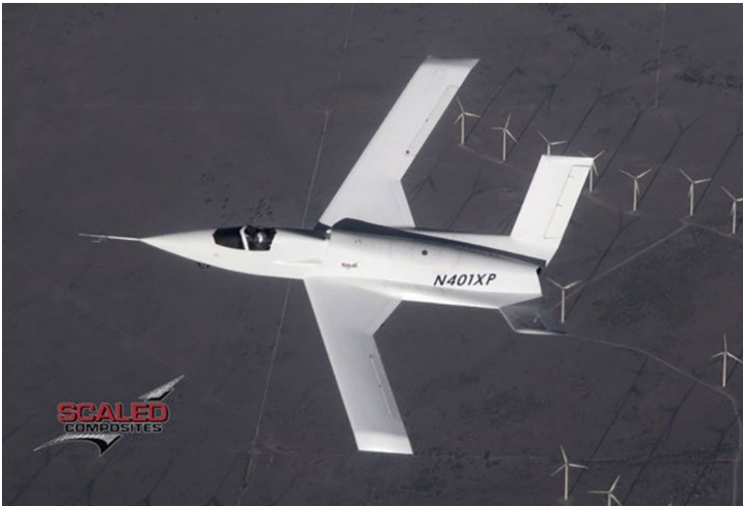
Model 401 design indicates several signature reduction features, including the dorsal engine and exhaust. Photo: Scaled Composites
