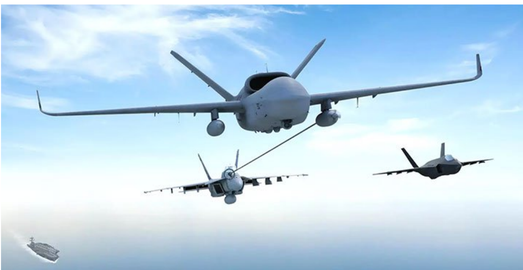
General Atomics is proposing a derivative of the Predator C Avenger for the US Navy carrier based unmanned refueling aircraft – Stingray. Photo: GA-ASI/USNI
