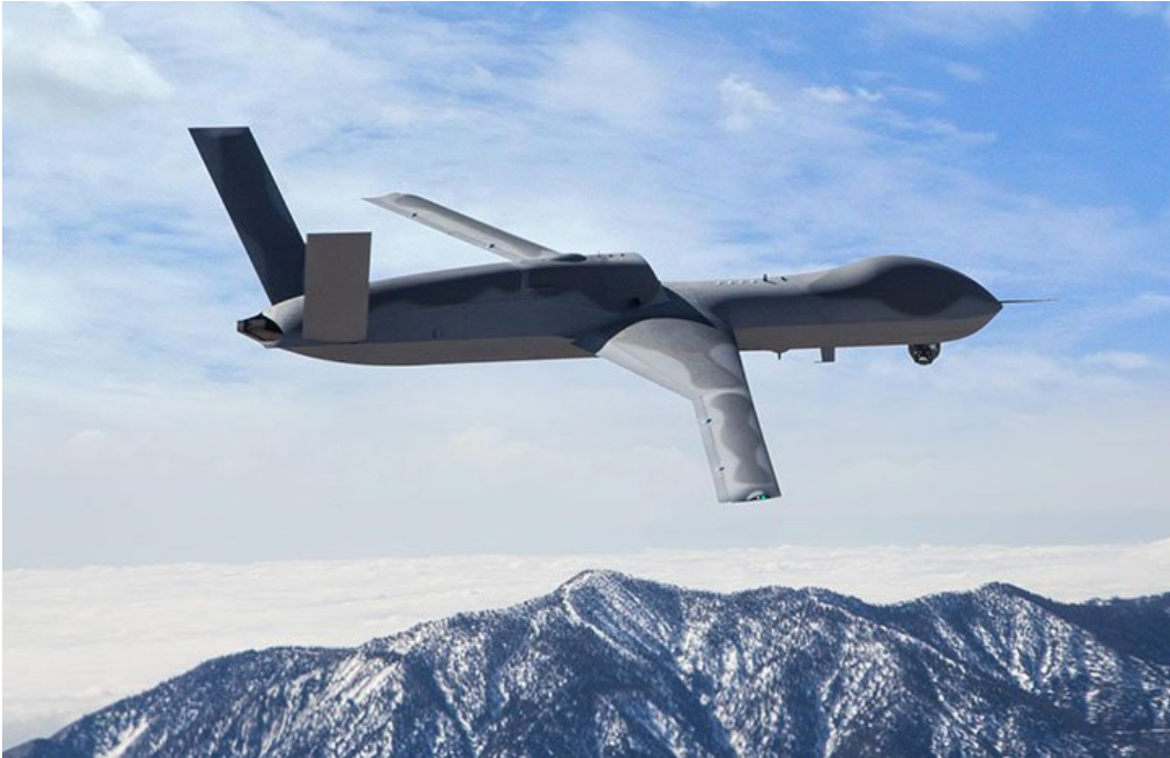
General Atomics' Predator C Avenger is a jet-powered unmanned aircraft that scales about three times larger than Model 401. The two vehicles are strikingly similar in their design features. Photo: GA-ASI
