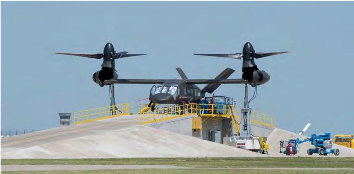
**Bell's V-280 is undergoing ground testing ahead of first flight in late October or early November. Credit: Bell Helicopter**
