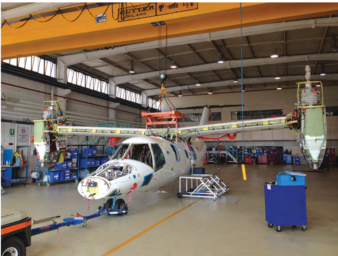
Protytype 3 is seen here being assembled in Italy. It is due to begin flight testing in Philadelphia, Pennsylvania, shortly.
