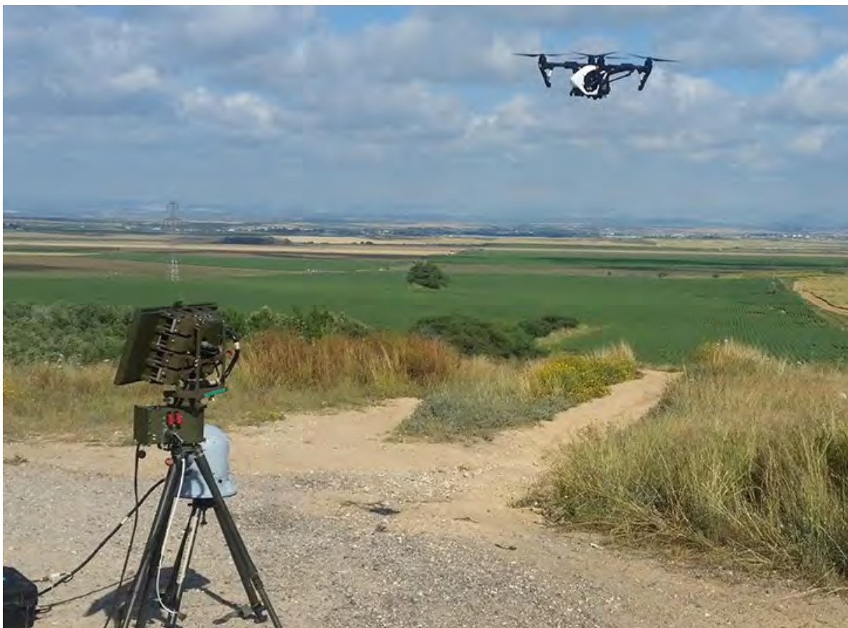
IAI Drone Guard Counter – UAS system comprises the ELM 3026 radar and electro-optical target recognition system, and an electronic jammer designed to disable the drone in flight., Photo: IAI
