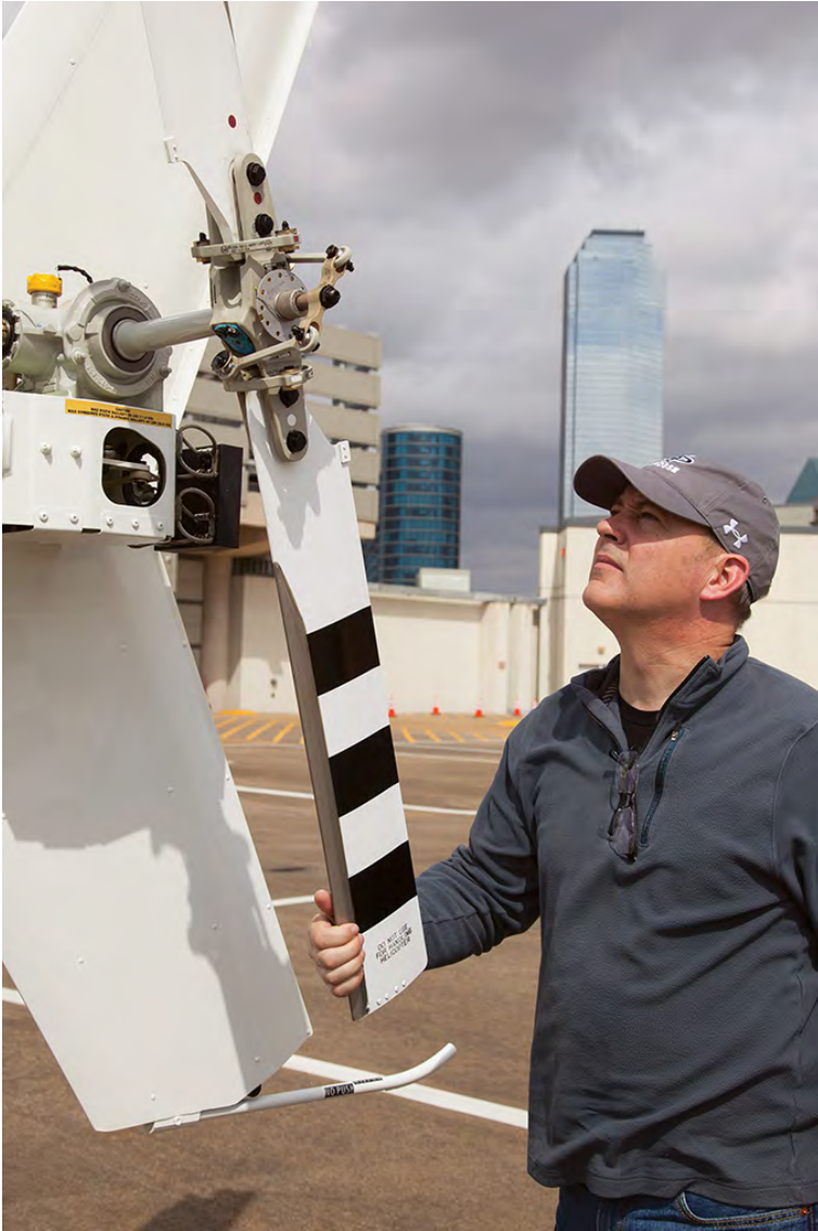
Bell's 505 Jet Ranger X retains the Model 206B's proven main and tail rotors and gearboxes. Credit: Tony Osborne/AW&ST
