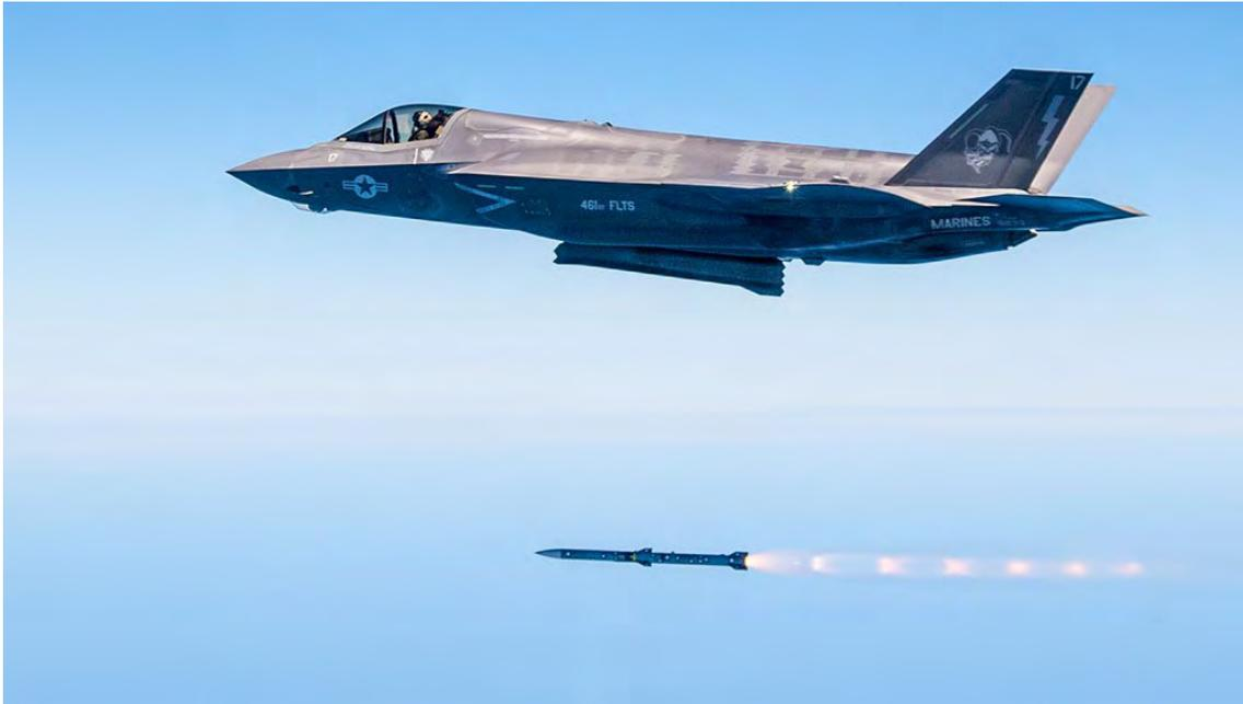
***An F-35B test pilot live fires an AIM-120 Advanced Medium Range Air-to-Air Missile (AMRAAM) above the Point Mugu Sea Test Range, California. This weapons test was one in a series of tests performed with the F35's latest 3F software in 2016. Photo: Lockheed Martin by Darin Russell.***
