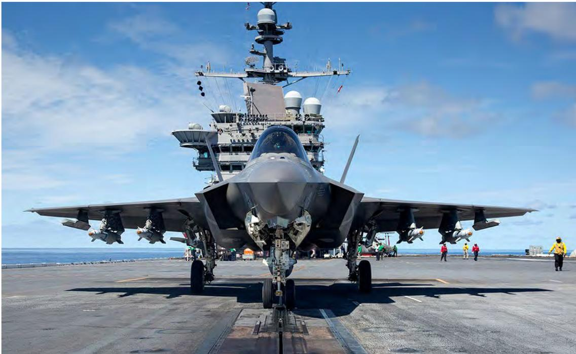
***The F-35C can carry weapons internally and externally. The wing is built with three hardpoints, two are designed to carry heavy weapons and the outer one is designed to carry lighter, air/air missiles.***
