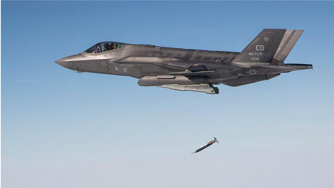
An F-35A drops a small diameter bomb during weapons tests. This weapons test was one in a series of tests performed with the F35's latest 3F software. Over the 31 calendar day "surge" period, the team accomplished 30 weapon releases (live fires and separations). Photo: Lockheed Martin by Chad Bellay
