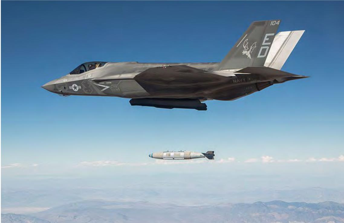
***An F-35C drops a GBU-31 Joint Direct Attack Munition (JDAM) bomb over China Lake Weapon Impact Range, California. This weapons test was one in a series of tests in 2016, performed with the F35's latest 3F software. Lockheed Martin photo by Chad Bellay.***
