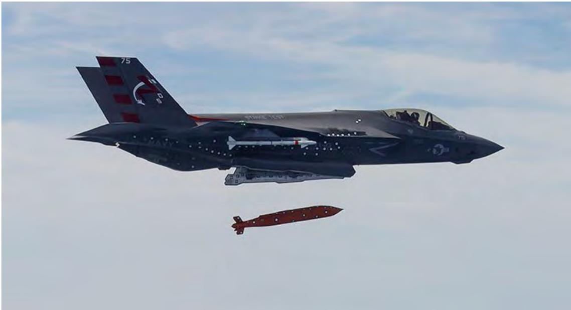
*The F-35 Lightning II Pax River Integrated Test Force from Air Test and Evaluation Squadron (VX) 23 conducted the first weapons separation test of an AGM-154 Joint Standoff Weapon (JSOW) from an F-35C Lightning II carrier variant March 23, 2016. Testing of the weapon revealed issues with mission planning and pilot-vehicle interface that limit the weapon's usability. Photo: U.S. Navy, by Dane Wiedmann.*
