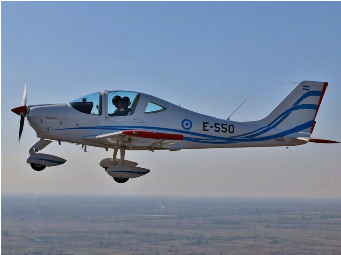
Tecnam P2002JF is a twin-seat trainer aircraft developed by Costruzioni Aeronautiche Tecnam for basic pilot training needs. The aircraft can also be used for surveillance and personal transportation missions.
