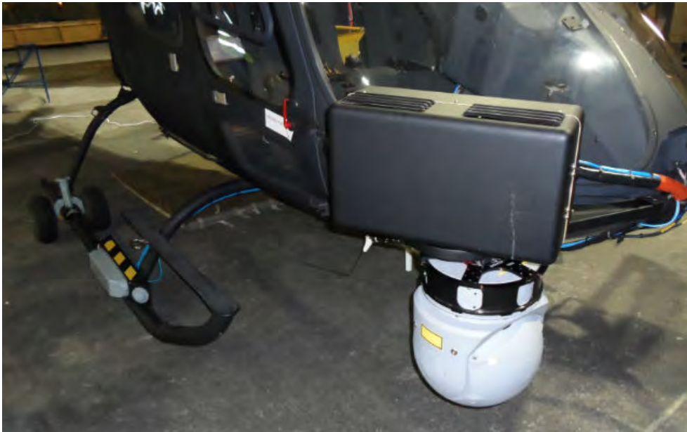
Solo carries skid-mounted Sage ESM and Osprey AESA radar (Beth Stevenson/FlightGlobal)
