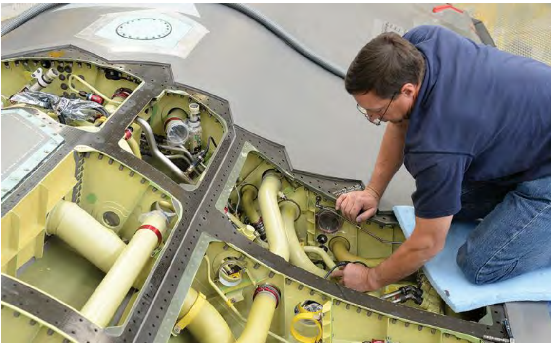
A maintainer at Hill AFB, Utah, works on an F-35. Credit: Hill AFB.
