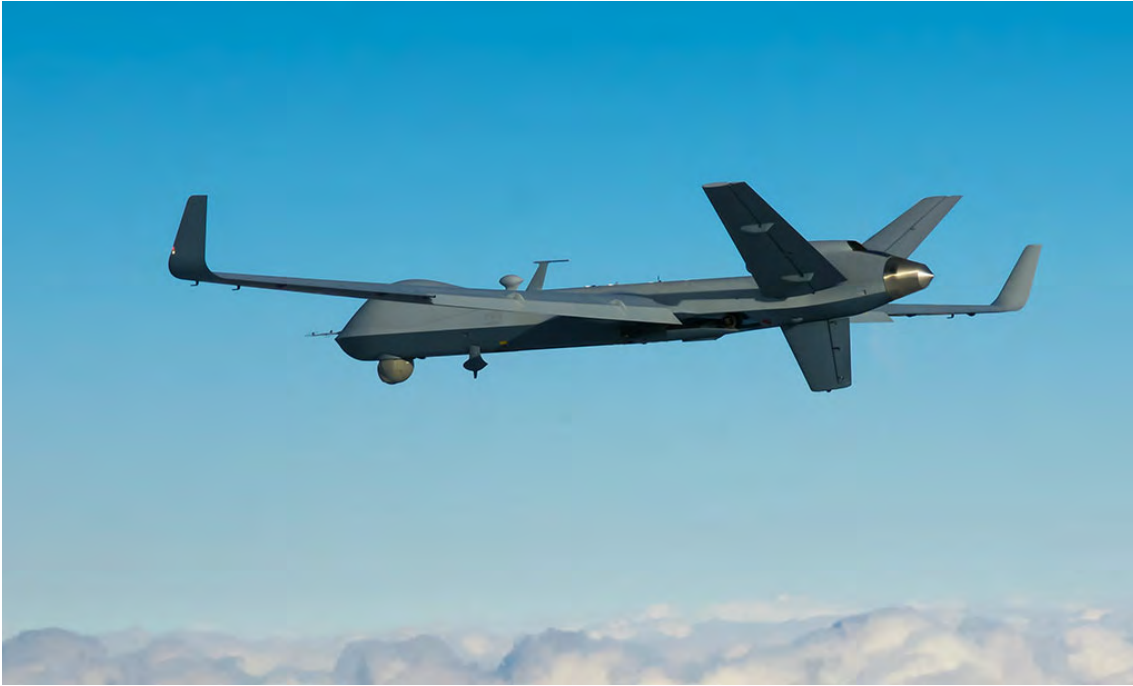
The ER variant of the Predator B (Reaper) flew in February 2016. It is equipped with longer wings and carries more fuel to extend mission endurance up to 40 hours. Photo: GA-ASI
