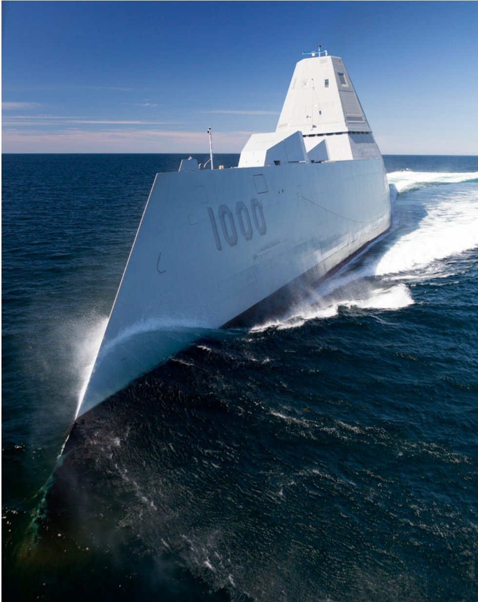
The 610-foot, wave-piercing tumblehome ship design provides a wide array of advancements. The shape of the superstructure and the arrangement of its antennas significantly reduce radar cross section, making the ship less visible to enemy radar at sea. Photo: US Navy
