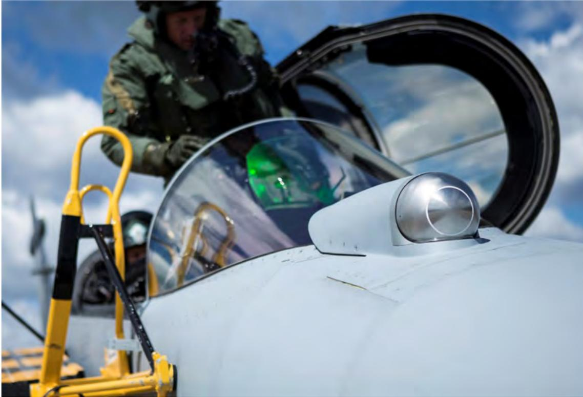
*The Skyward IRST enables Gripen E pilots to track and engage targets without giving away their positions. Photo: Saab*
