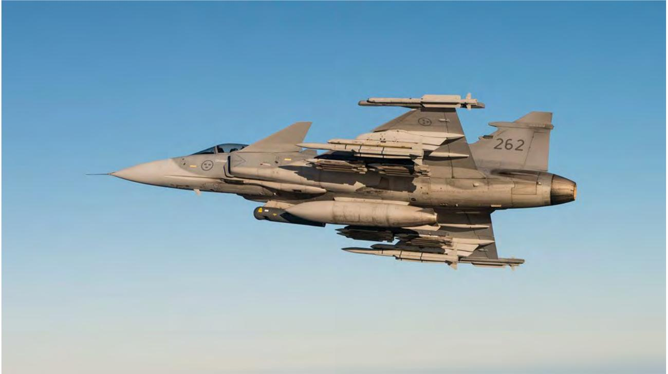
**SAAB Gripen C carrying a weapon configuration including eight GBU-39 Small Diameter Bombs, two Meteor and Two IRIS\_T Air/Air missiles. The aircraft also carries a fuel tank on the centerline, Litening targeting pod and an internally mounted 27mm Mauser cannon. Photo: SAAB**
