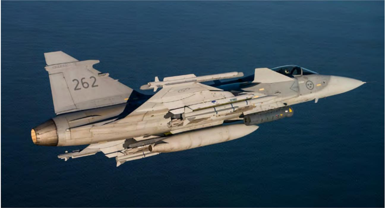
*Saab Gripen C fighter armed with air/air and air/ground weaponry. Photo: Saab*
