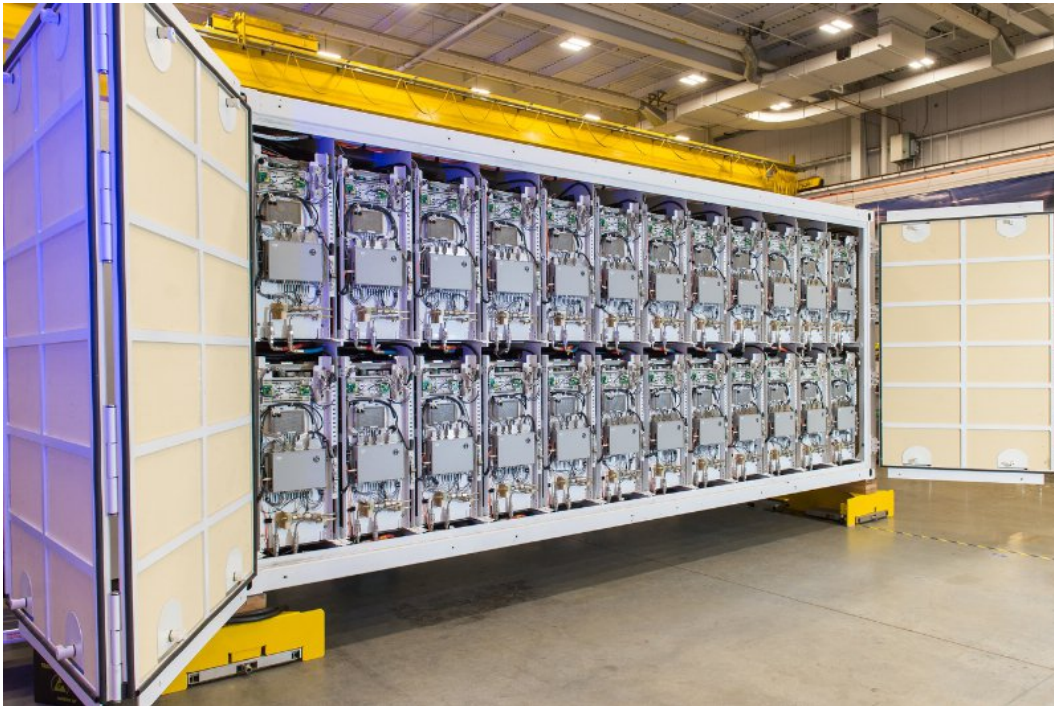
Raytheon has completed the first examples of containerized pulse power packs designed to support field tests of the electromagnetic rail gun. Photo: Raytheon.
