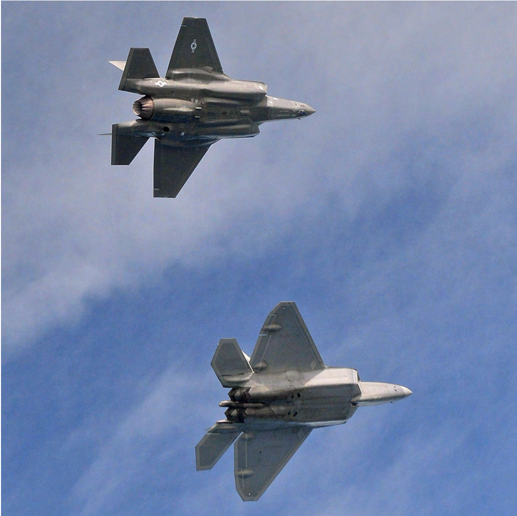
The underside of the F-22 is much flatter than that of an F-35. Photo by MSgt. Shane A. Cuomo
