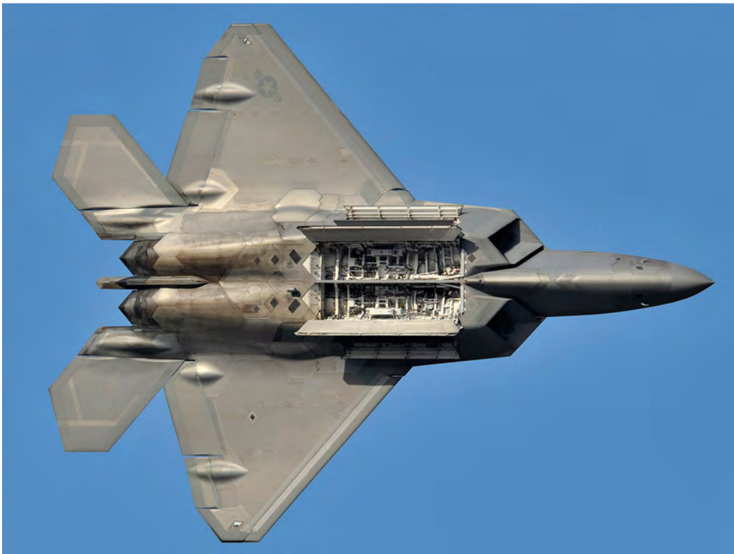
The F-22 has one main (though split) weapon bay with two doors. The F-35 has two distinct main weapon bays each with two doors. Top Photo by Andy Wolfe ; Bottom Photo by Katsuhiko Tokunaga
