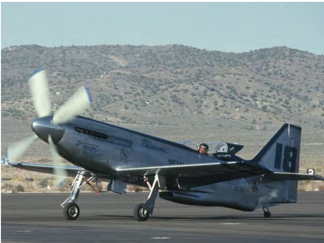
Tsunami looked like a warbird and had the power of the 1940s fighters it was built to replace: It used the same Rolls-Royce V-12 Merlin engine. (Robert F. Pauley)
