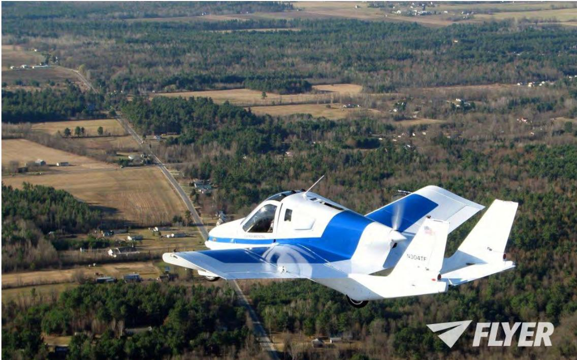
***The Terrafugia Transition flying car has been allowed a weight increase to 1,800 pounds (816kg) to allow it to include car-type safety features.***
