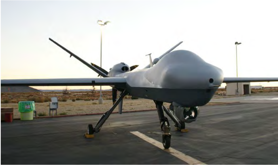
The mounted system DAA being tested included a Due Regard Radar (DRR) developed by the company, Honeywell's Traffic Alert and Collision Avoidance System (TCAS) and Sensor Tracker, specifically designed for DAA. Photo: GA-ASI
