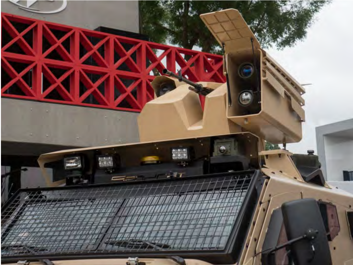
The Samson RWS integrates a heavy machine gun, two Spike LR missiles and optronic system. The vehicle is also fitted with Spotlite M IR hostile gnsht detection system and panoramic cameras. Photo – Noam Eshel, Defense-Update
