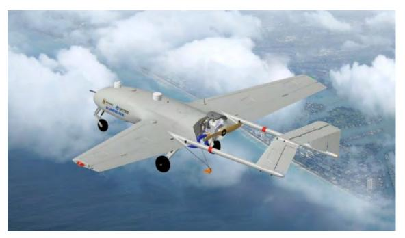
The new tactical drone developed by Korean Air has a length of 3.4 meters and a wingspan of 4.2 meters. It is designed for short, automatic takeoff and landing, deploying from a short runway of 30 meters, and landing on wheels, skids, or parachute. Photo: Korean Air
