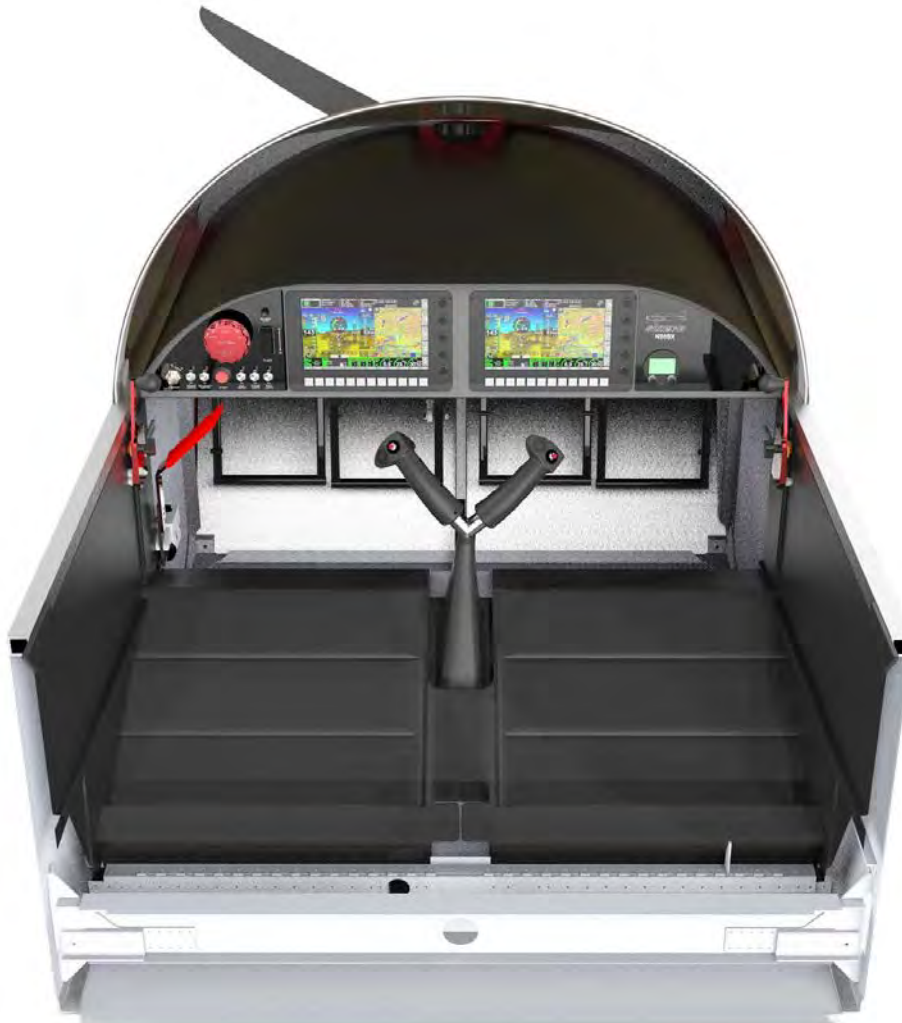
View of the new Sonex B-Model seating and panel, wider than before.
