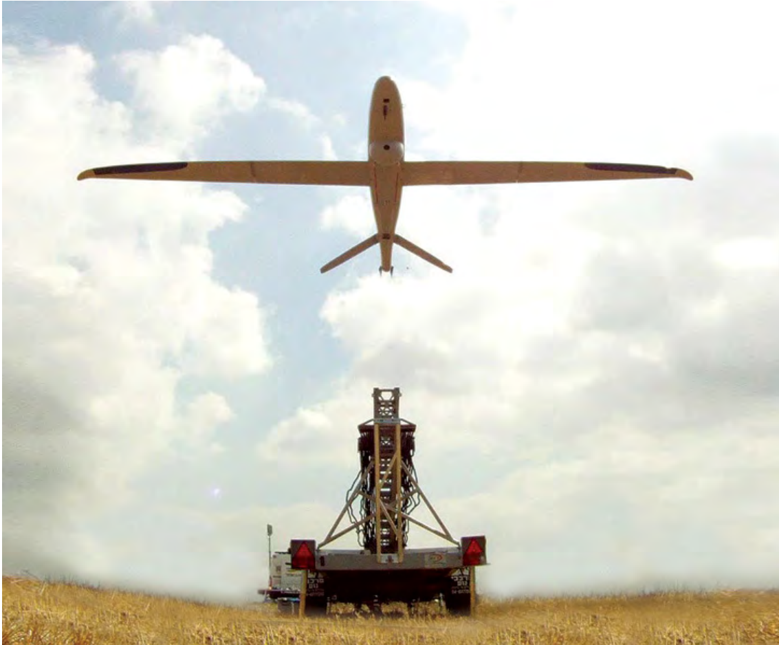
Launched via a pneumatic launcher, mounted either on the ground or on a vehicle, Skylark 3 offers upgrades such as improved payloads with better target detection, classification and surveillance capabilities. Photo: Elbit Systems
