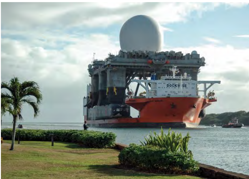
The Sea-Based X-Band radar, the world's largest phased-array X-band system, travels on an oceangoing oil platform and is able to distinguish decoys from warheads. (Ryan C. McGinley/US Navy)
