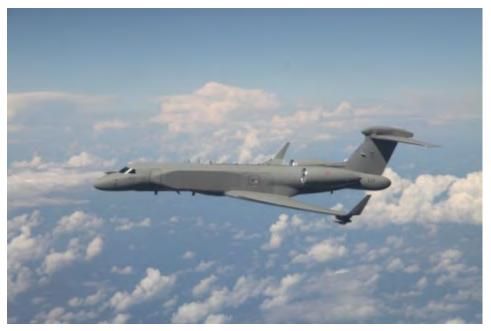
The first G550 Conformal AEW aircraft in Italian Air Force markings. It fitted with conformal radar antennas allowing 360-degree coverage, and a wide range of sensors. A second aircraft is due to follow in 2017. (IAI photo)
