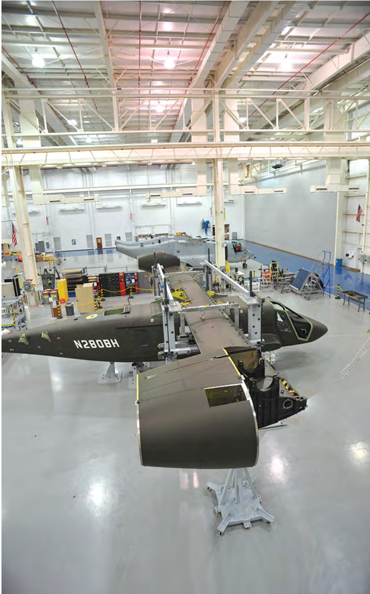
The V-280's engines will be installed in the fixed nacelle structures that are already mated to the carbon-fiber wing. Credit: Mike Calcote
