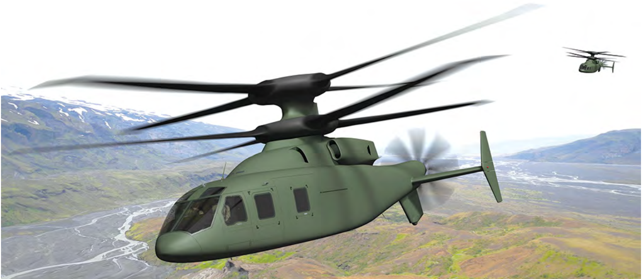
SB-1 scales up Sikorsky's X2 coaxial rigid-rotor configuration to the 30,000-lb. class. Credit: Boeing
