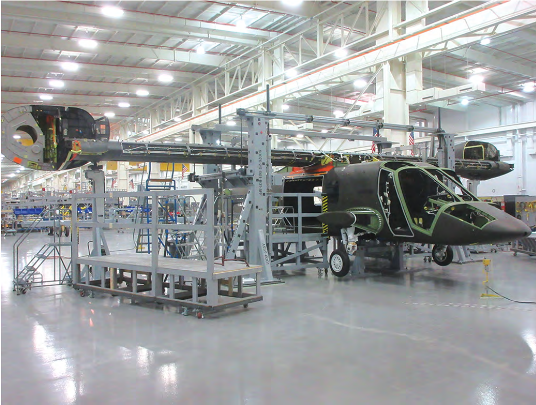
A Bell Boeing V-22 is in the background as the V-280 goes through wing mating in Amarillo, Texas. Credit: Mike Calcote/Textron Photos
