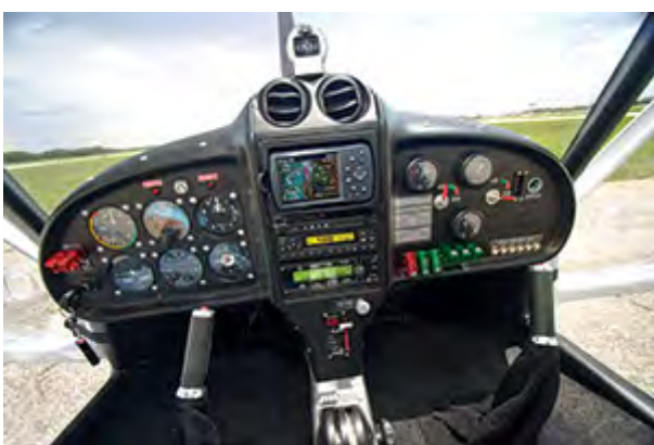
The fully equipped MD3 Rider features steam gauges and Garmin electronics. The electric-flap lever (below) is easily reached and user-friendly.
