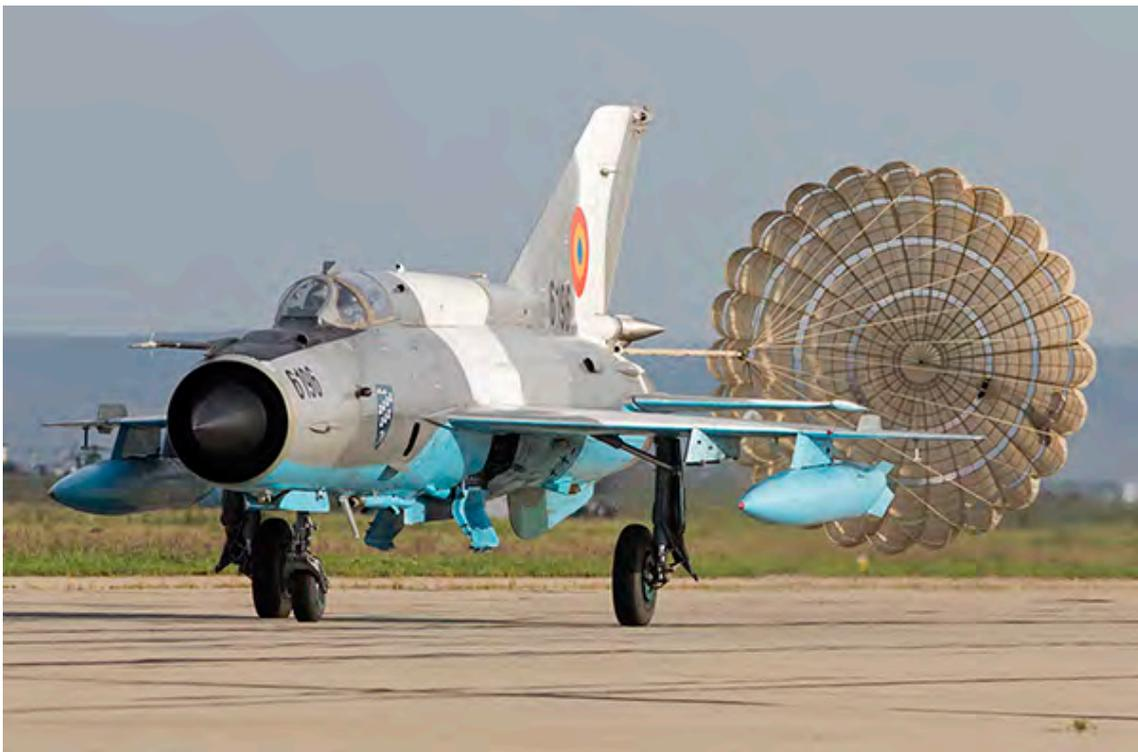
**Brake parachutes are needed with a landing speed of 190 kts.**
