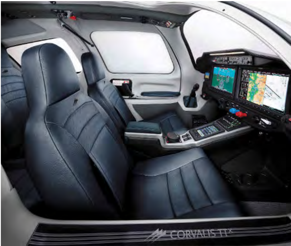
The side-stick arrangement makes the cockpit feel even more spacious. Textron Aviation Photo
