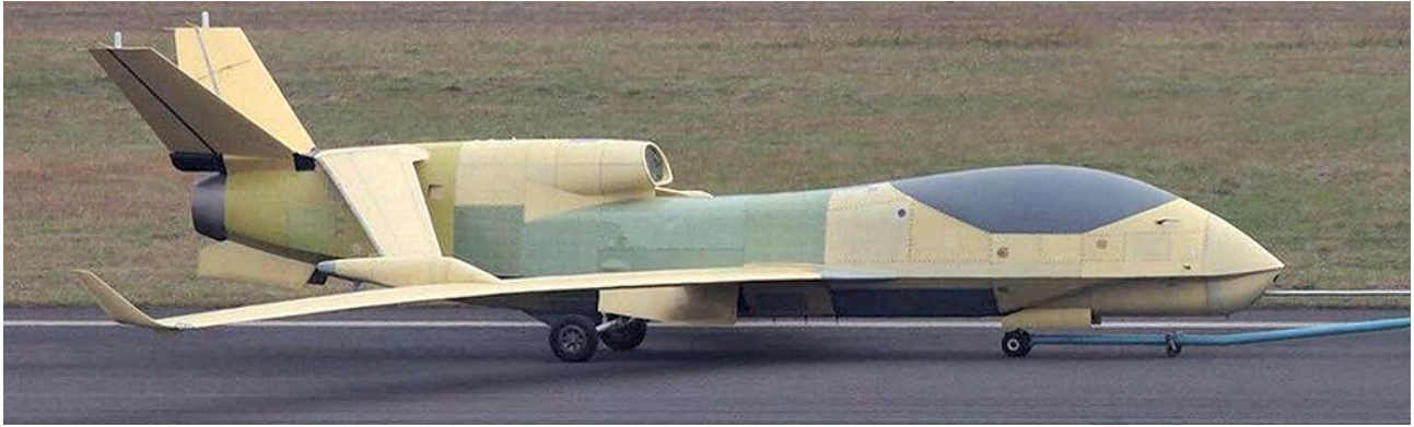
Joined-wing Soar Dragon could be capable of high subsonic speeds. Credit: Chinese Internet
