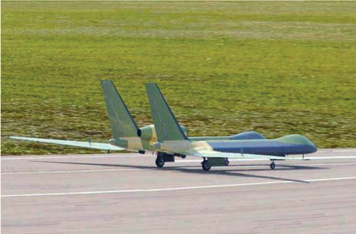
The outer half of each of the Divine Eagle's twin bodies appears to be a radome. The total vertical tail area is strikingly large.
