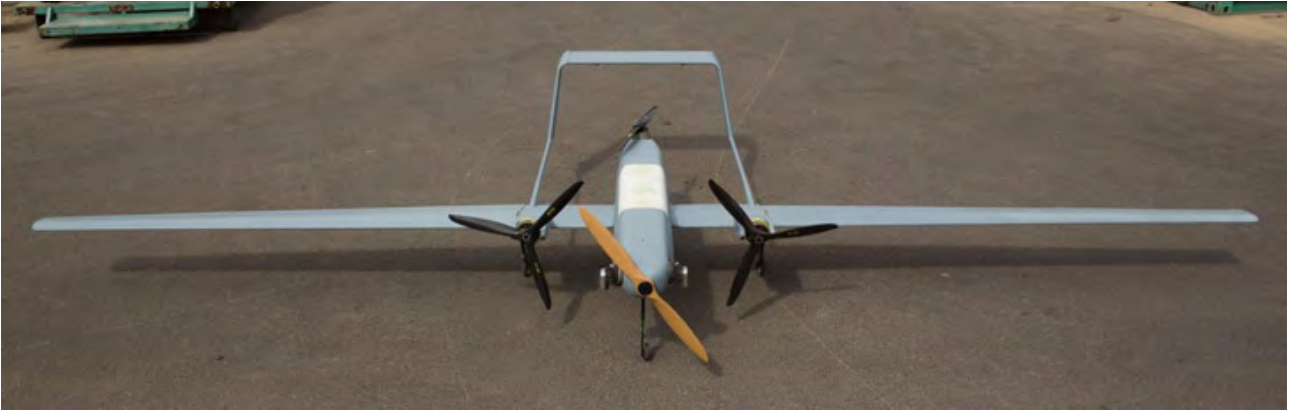
At 67 kg of weight, FE Panther weighs only two kilograms more than the all-electric Panther launched by IAI in 2010. Photo: IAI
