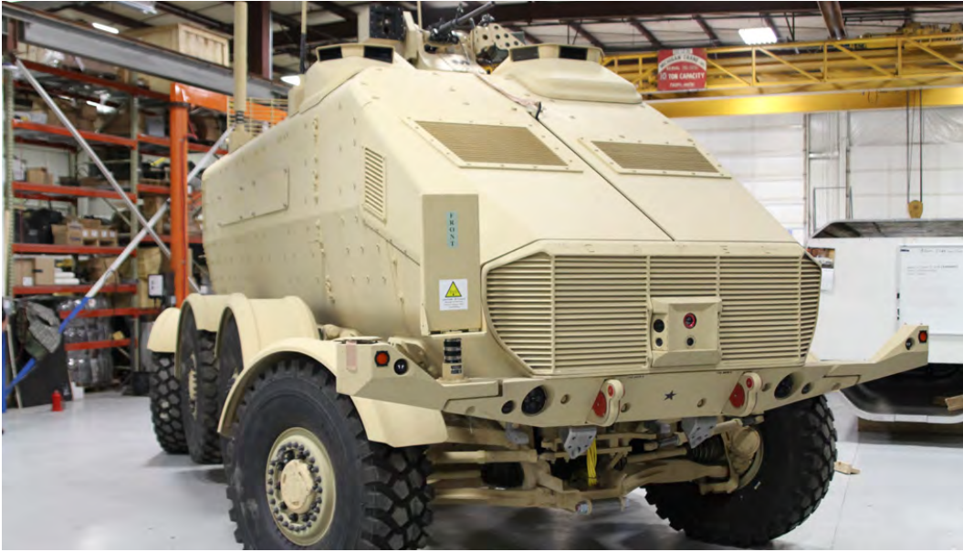
The CAMEL concept vehicle demonstrator is shown here with its carriage, peripheral cameras, and C-IED devices adding to the vehicle's protection. Photo: US Army
