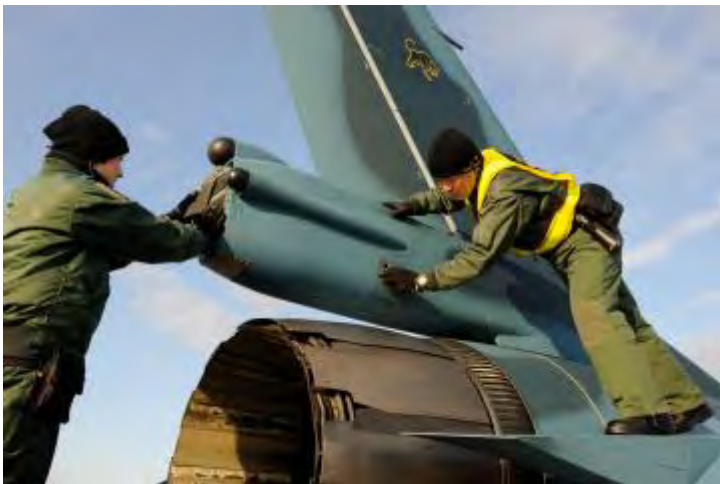
All F-2s carry a drag chute for landing. The chute is used regularly in icy conditions common in Japanese winters. Photo by Ito Hisami
