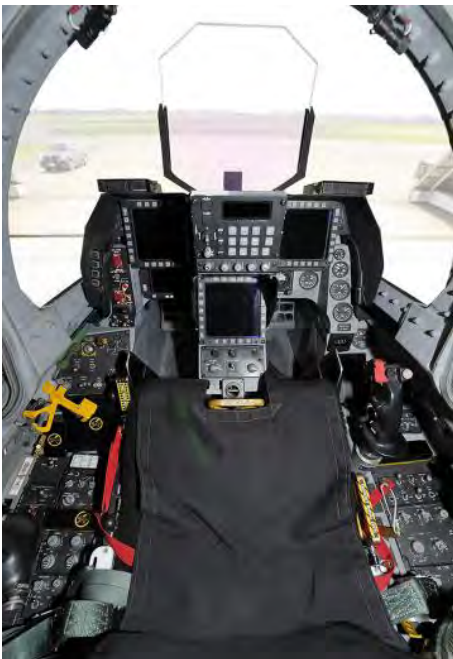
The F-2 is the first fighter aircraft in JASDF that adopted a glass cockpit. The F-2 cockpit has three full color multifunction displays showing radar, weapon information, terrain map, and electronic warfare information. The control stick is on the side of cockpit as in the F-16, F-22, and F-35. Photo by Katsuhiko Tokunaga
