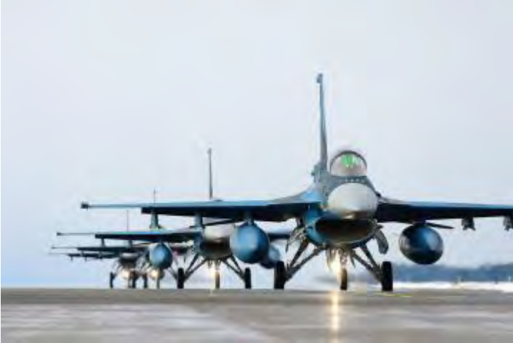
The F-2 incorporated a number of new technologies for its time. For example, it was the first production fighter to be equipped with an active electronically scanned array radar. The wings on the F-2 are made of fifty-five percent composite material by weight. Photo by Ito Hisami
