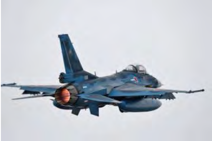
The F-2 is powered by a single General Electric F110-GE-129 engine, which produces more than 29,000 pounds of thrust. Photo by Ito Hisami
