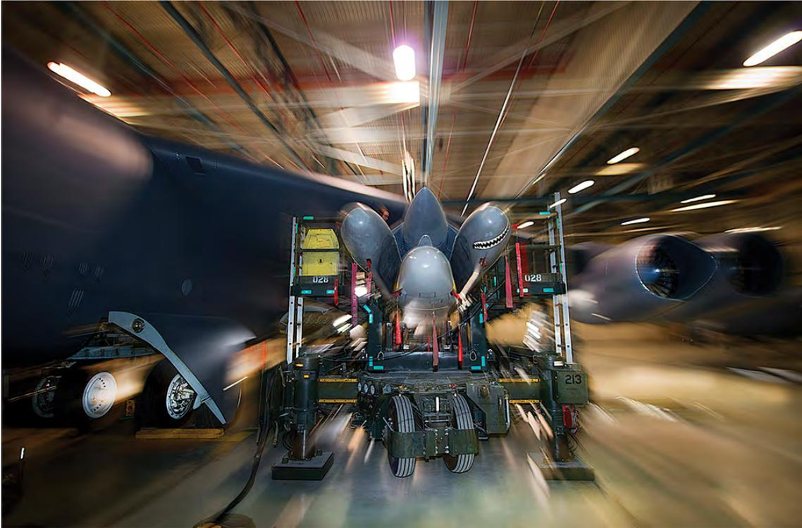
***The B-52H can carry a total of 20 AGM-86B air-launched cruise missiles with W80-1 nuclear warheads on its wings and internally. Here, crews load ALCMs onto a “Stratofortress” bomber at Minot AFB, North Dakota. Credit: U.S. Air Force***
