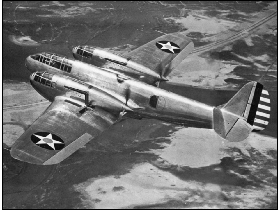
▲ This undated photo shows a YFM-1. Differences from the XFM-1 include flat panels in the cockpit canopy for less optical distortion, flush-mounted aft fuselage gun positions rather than teardrop blisters, no air intakes on the nacelle tops and no engine-driven turbo-superchargers—the dark “Z”-shaped stacks on the nacelles exhausted to plain turbos underneath the wing. The cannons and machine guns were not installed when this photo was taken.
