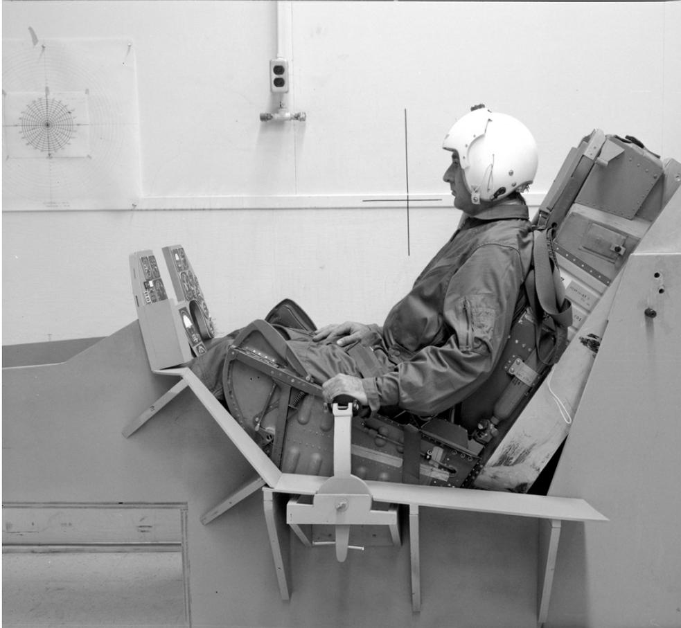
*The thirty-degree seatback angle and a raised heel rest line provided increased tolerance to g forces in the YF-16. Side-mounted stick and throttle controllers allowed for more precise control under high g's. Locating combat-critical functions on these side-mounted throttle and stick controllers further enhanced the pilot-vehicle interface for the high-g regime. The bubble canopy on the YF-16 design improved pilot vision for air-to-air combat.*
