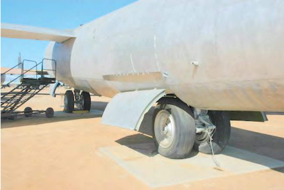
A close-up of the B-47's "bicycle" landing gear. Placing the landing gear in the the B-47's thin wings would have required drag-producing bulges. (Scott Schwartz)
