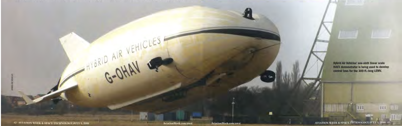
Northrop Grumman's LEMV will orbit unmanned for at least three weeks at 20,000 ft. carrying a 3,500-lb. payload of sensors.
