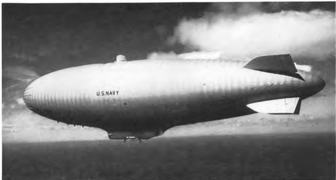
GOODYEAR ZPG-3W , airborne early warning airship, carries a 40 ft. search radar antenna within its helium envelope. Pod atop the airship contains height-finding radar. The 403 ft. blimp has an absolute ceiling of 10,000 ft. and a useful load capacity of 22,907 lb.
