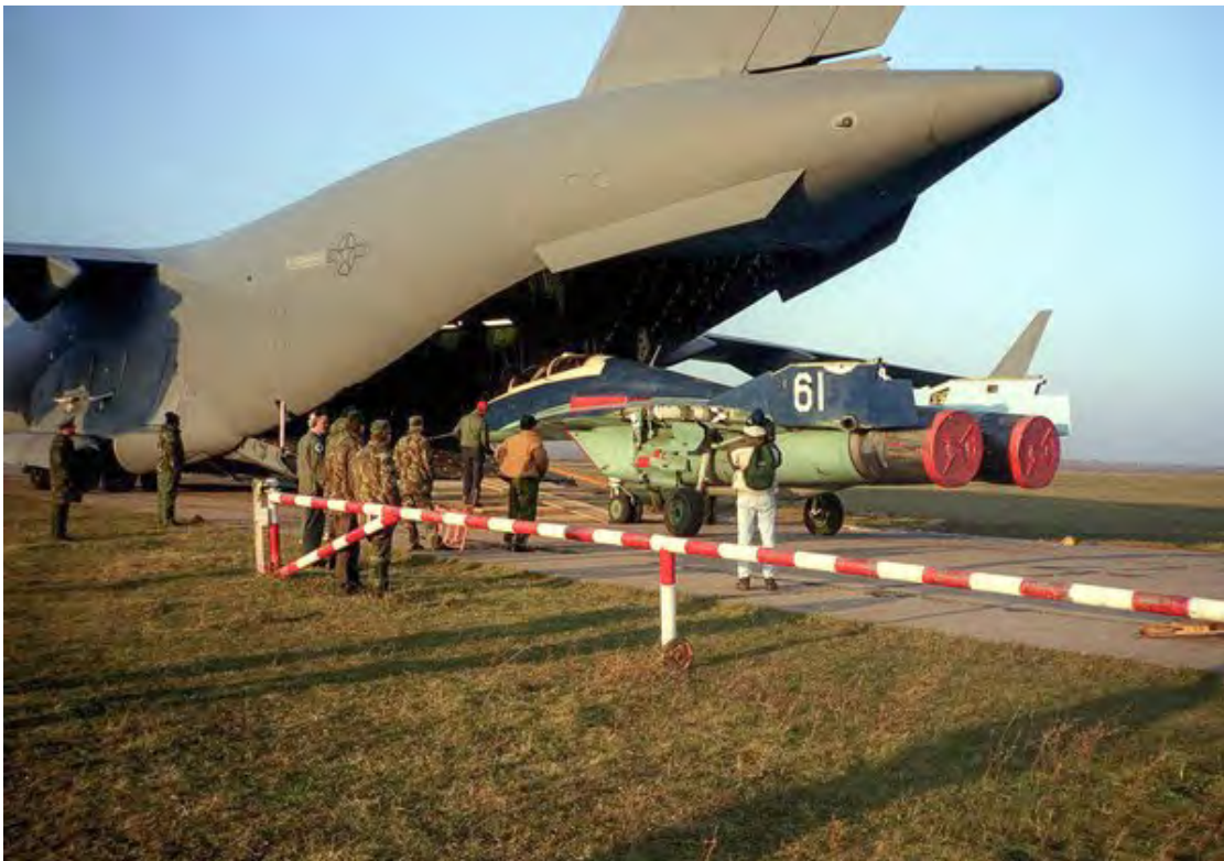
A MiG-29 trainer is winched aboard a C-17 for shipment from Moldova to the United States. (Department of Defense)
