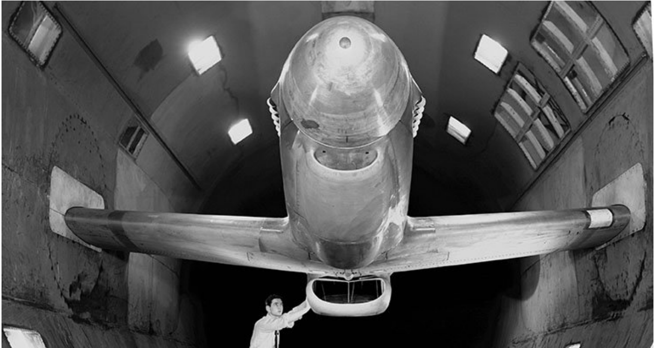
North American XP-51B Mustang in the 16 foot wind tunnel of the NACA Ames Aeronautical Laboratory, in March 1943, readied for full scale studies of duct rumble.
