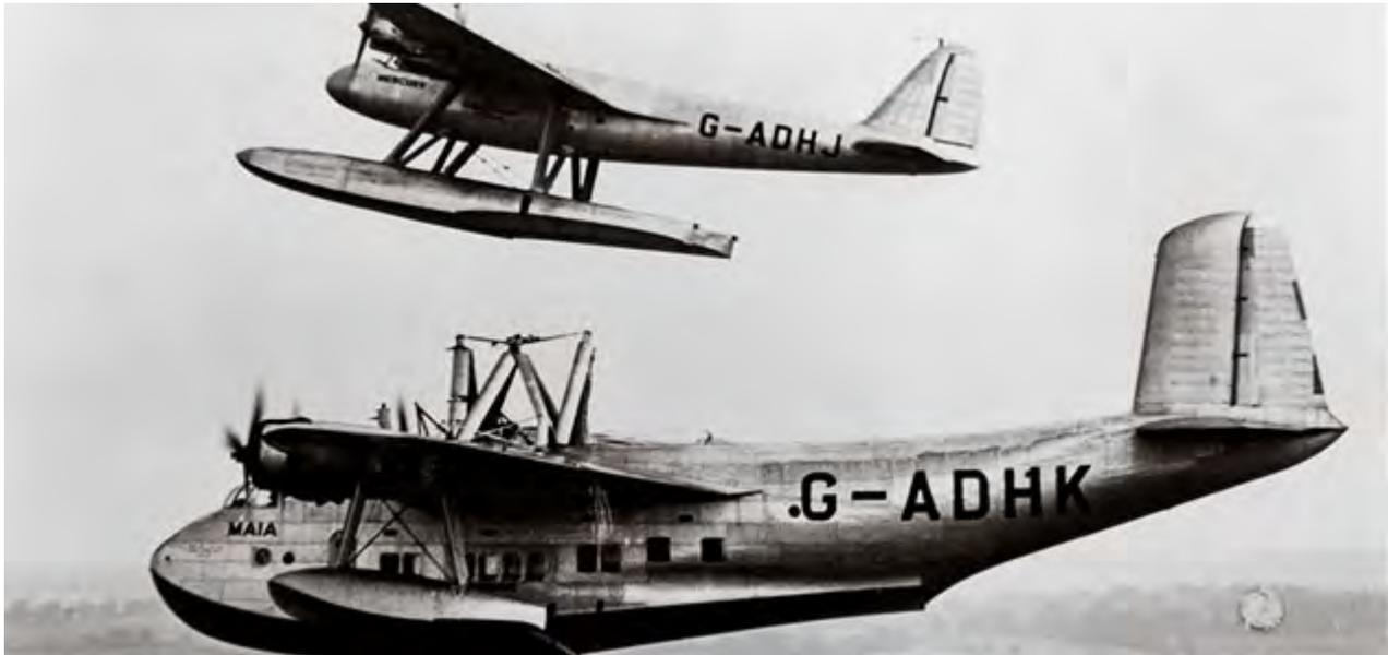
**The S.20 Mercury pulls away from its launcher aircraft, the S.21 Maia, at the start of the pair's 1938 nonstop flight.**
