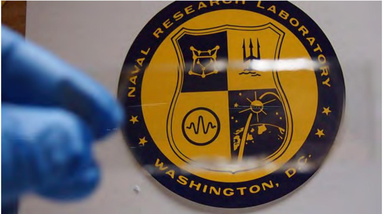
***The NRL-developed transparent polymer armor consists of alternating layers of elastomeric polymer and a harder material substrate. Very small crystalline domains, which also provide rigidity, give the polymer its transparency. Photo: US Navy/NRL***
