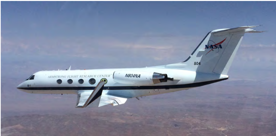
One tech demo successfully completed tests of flaps that can be changed to different angles during flight, reducing drag and noise. Photo: NASA
