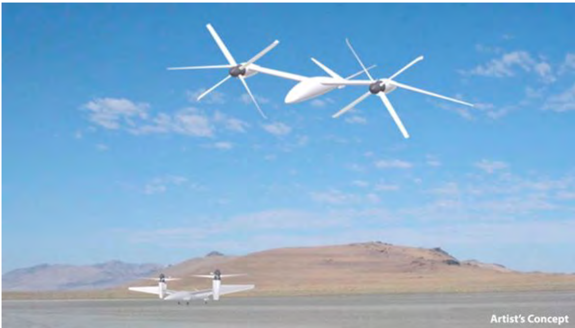
Karem's TR36XP's proprotor will improve efficiency in both modes by dramatically changing its rotation speed. (Karem)
