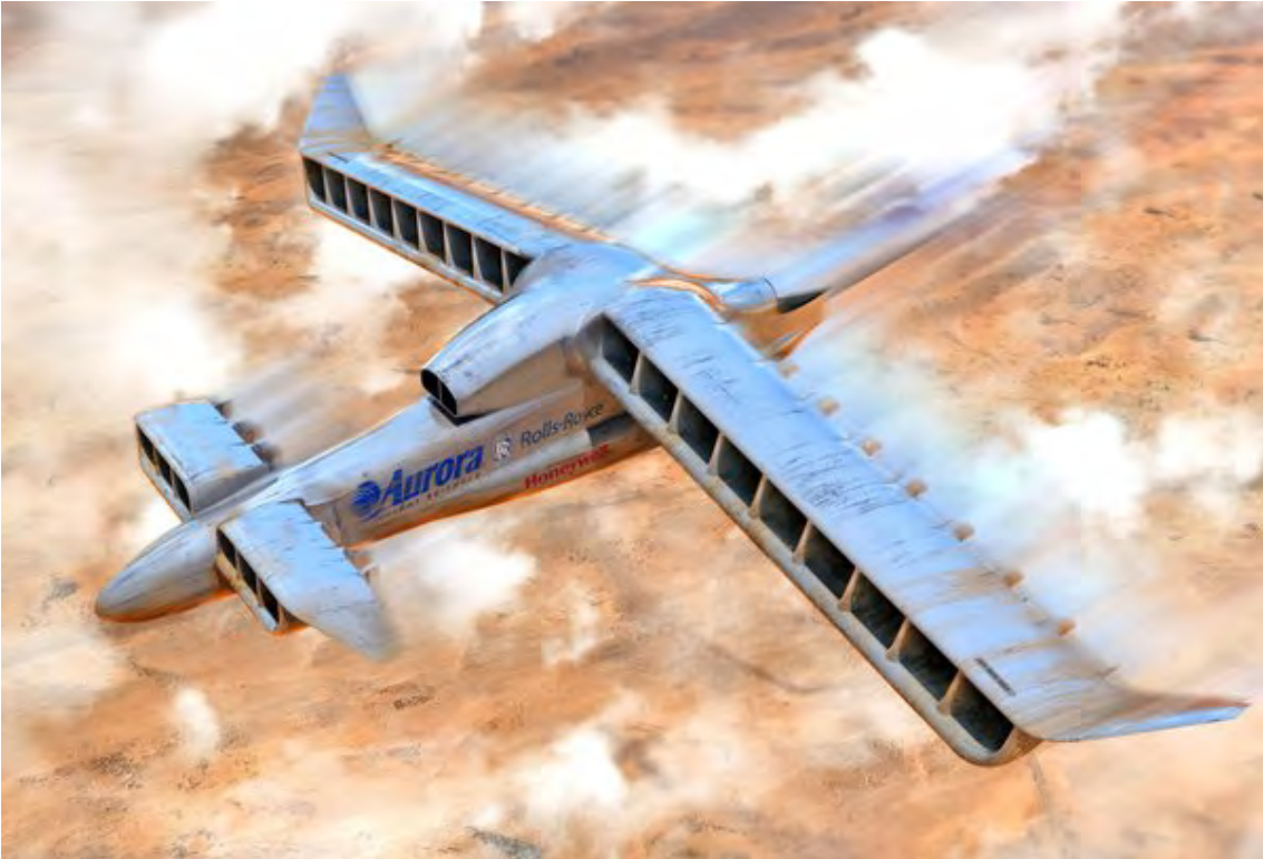
Aurora Flight Sciences' entry (shown here in an artist's conception) tilts the entire wing—and the motors with it—much like the Vought XC-142 used to do. (Aurora)
