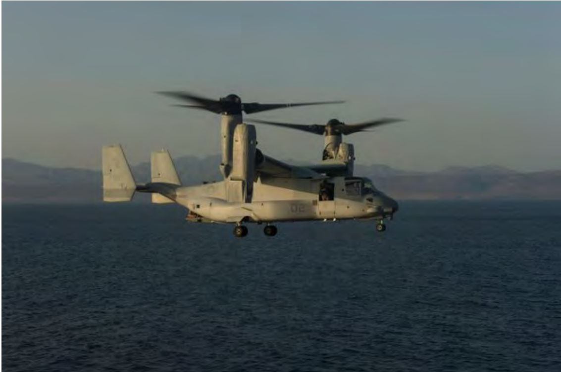
The V-22's proprotor blades are short and twisted, a compromise between forward and vertical flight. (U.S. navy/Kenan O'Connor)
