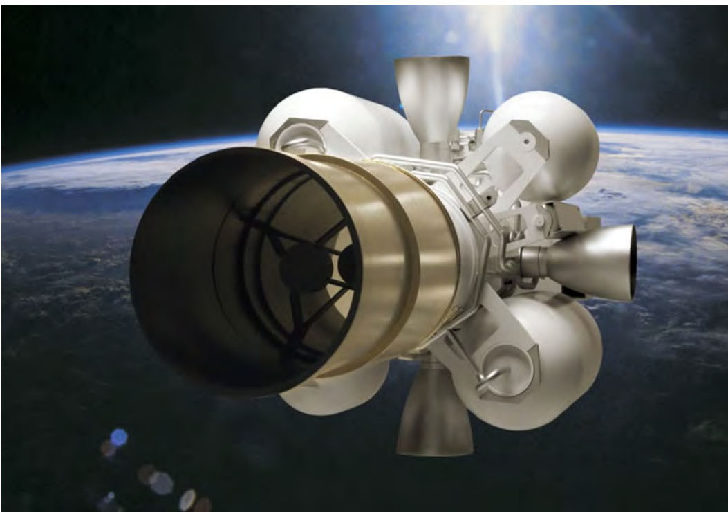
Raytheon's Exoatmospheric Kill Vehicle (EKV) is the intercept component of the Ground Based Interceptor (GBI). Illustration: Raytheon
