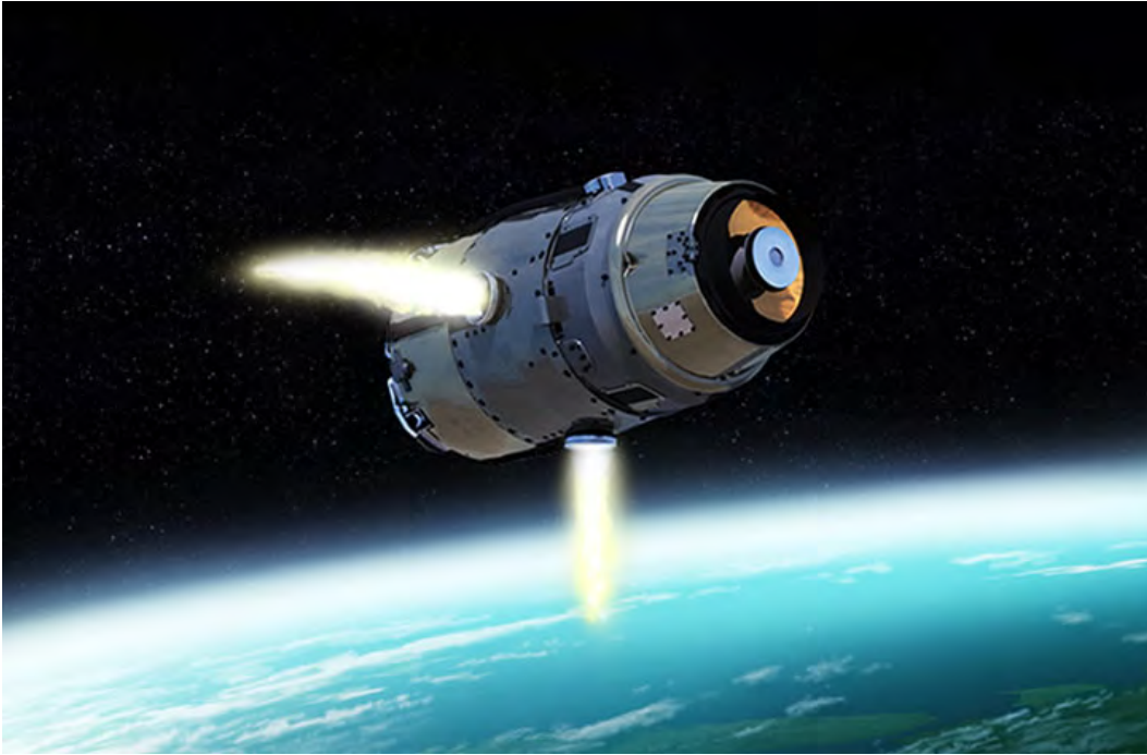
The SM-3's exoatmospheric vehicle collides with its target to obliterate the threat without the need for explosives. The resulting impact is the equivalent to a 10-ton truck traveling at 600 mph. Illustration: Raytheon
