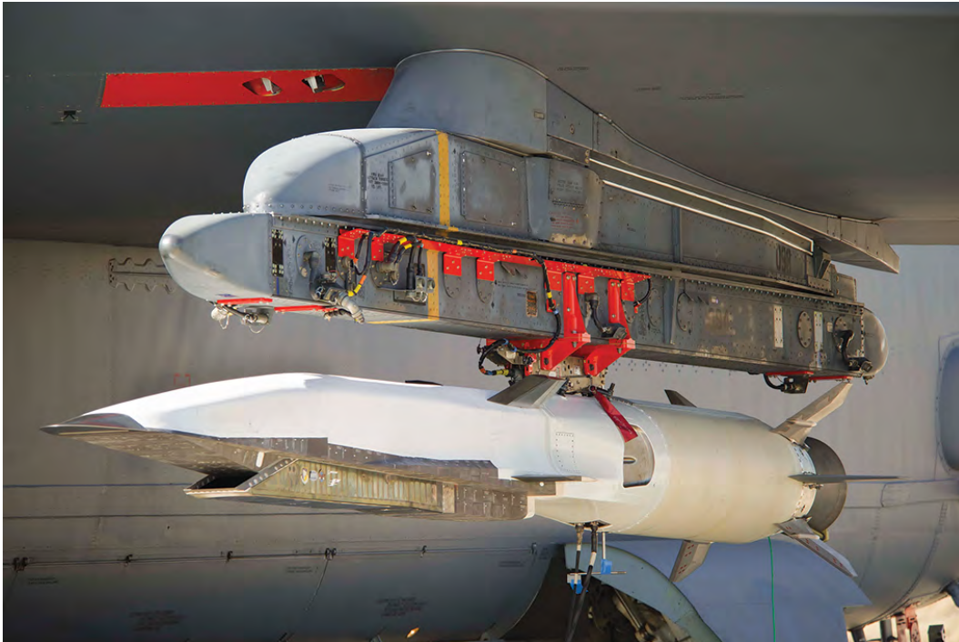
Boeing's X-51A was powered by a fuel-cooled, kerosene-fueled scramjet. Credit: U.S. Air Force
