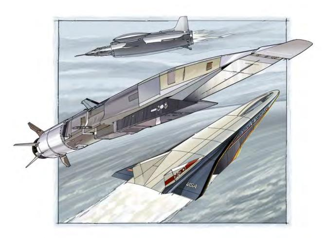
Engineers have been experimenting with ramjets since the 1930s. From top: The French Leduc 0.10, test flown in 1949; the Boeing X-51 Waverider, which flew in 2009; the Rockwell X-30 NASP, cancelled before it could fly. (Illustration by Harry Whitver)
