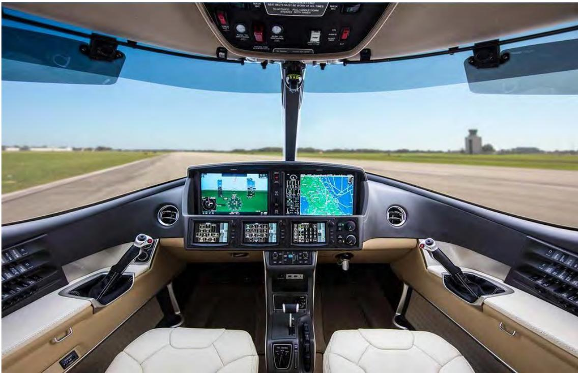
*The Vision's sidestick is linked to the control surfaces by pushrods, and lacks the spring loading of the SR series' sidestick for a more natural feel in flight.*
