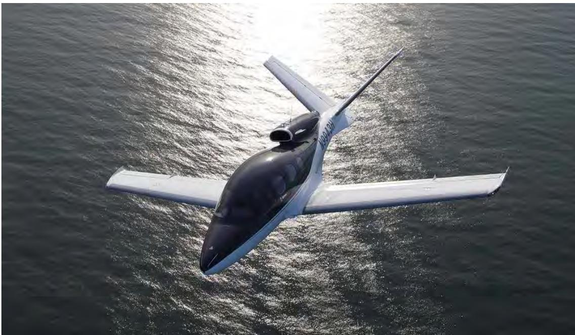
*The Vision, with its single Williams FJ33-5A turboprop sitting atop the fuselage, is an aerial curiosity that will take some time for ATC to figure out. It performs more like a turboprop than a turbojet airplane.*
