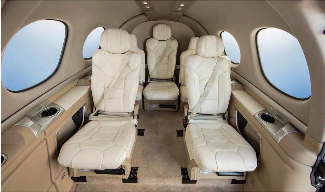
*There's room for seven inside the Vision Jet, which features seats that can quickly be removed or rearranged to customize the cabin to fit your needs. You won't be able to fill all the seats with people and top the fuel tanks, but at max gross weight range is still a respectable 500 nm flying at max continuous thrust. The SF50's performance sweet spot is 800 pounds of payload, providing roughly 800 nm of range.*
