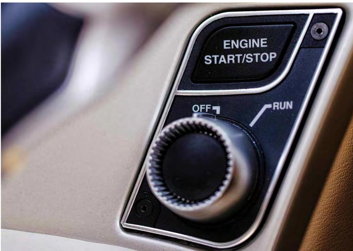
*The engine start sequence in the Vision is a no-brainer. Turn the dial to "Run," press the "Start" button and let the computerized faDEC handle the rest.*
