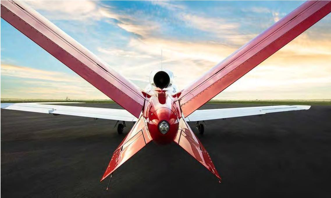
*V tails can offer aerodynamic advantages, such as cruise speeds higher than those with conventional tails and better resistance to spins. They can also exhibit a tendency to hunt around in yaw if not flown carefully. The Vision Jet overcomes this with the use of a yaw stability augmentation system built into the lower ventral fins that automatically cancels out dutch roll to provide a smooth and efficient ride.*
