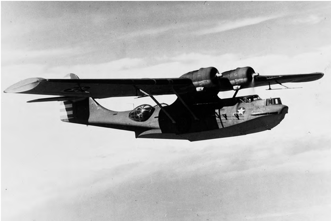
This PBY-5A shows off some of the Catalina's attributes, long "wet" wings, bulging waist gun positions and dipole radar antennas under each wing. (U.S. Navy)
